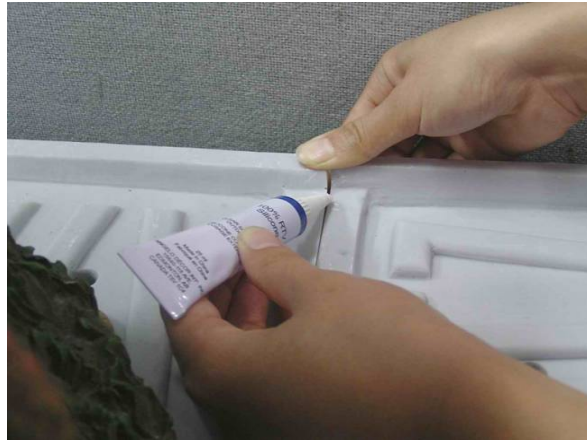
Install pump access door. Using tube provided, apply silicone along seams. Add decorative rocks on top of tray.
